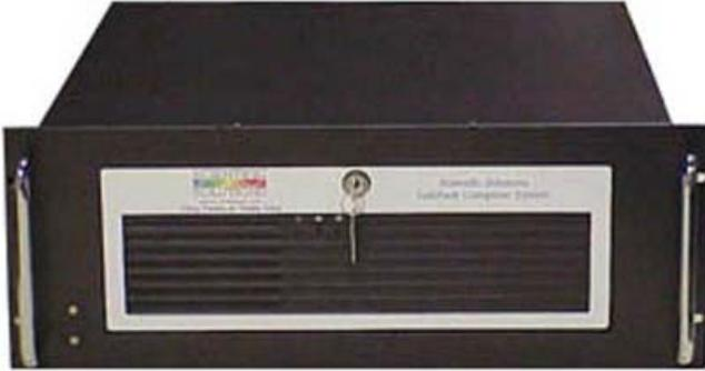
The LabRack Computer System contains the Scientific Solutions LabMaster data acquisition system. This is the brains of the tester and is responsible for the control signals and the monitoring and acquiring of the data.
